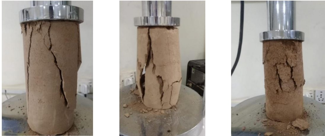
Figure 4-11 :Failure of the Sample in Unconfined Compression Testing.
