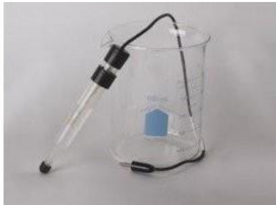
Figure1.18: Illustration of Ag/AgCl reference electrode
