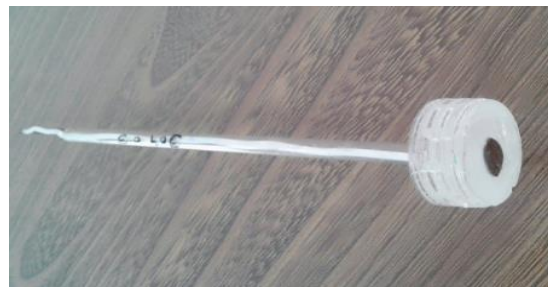
Figure 3.5: Image of cold mounted electrode
