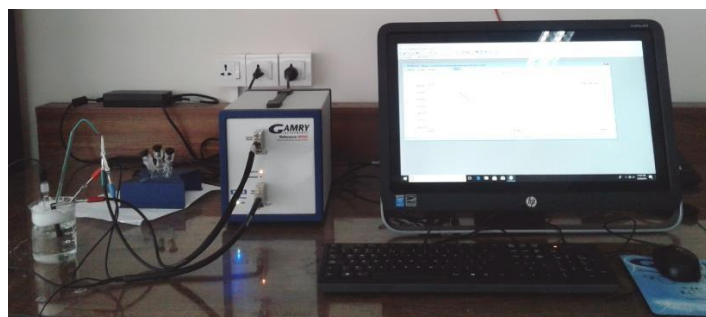
Figure 3.7: Demonstration of Gamry potentiostat
