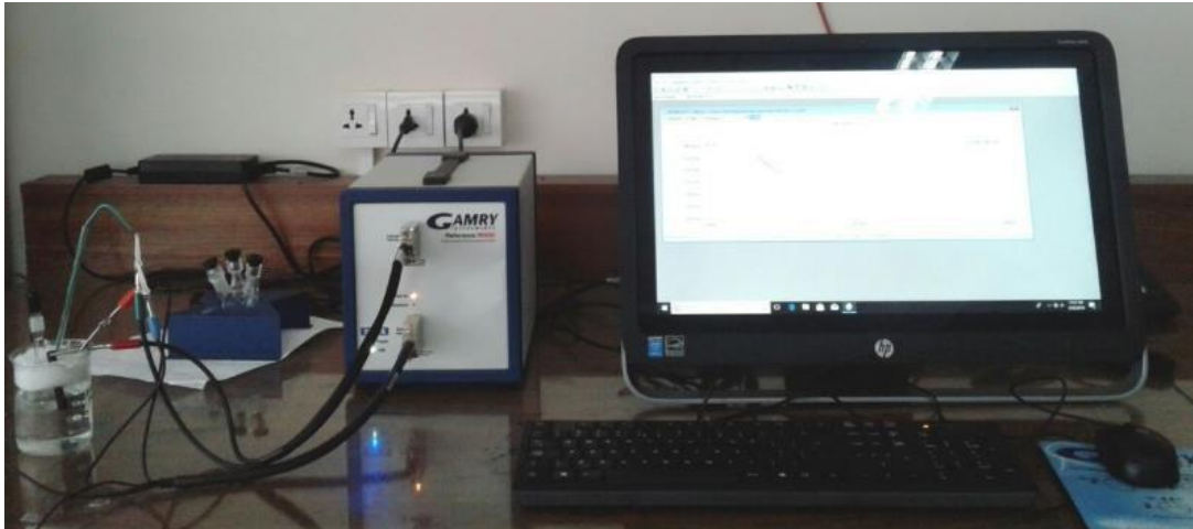
Figure1.17: Demonstration of Gamry potentiostat/Galvanostat/ZRA
