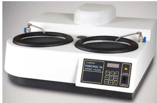
Figure 3.2: Image of grinder and polisher
