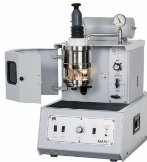
Figure 3.1: Illustration of Arc melting furnace
