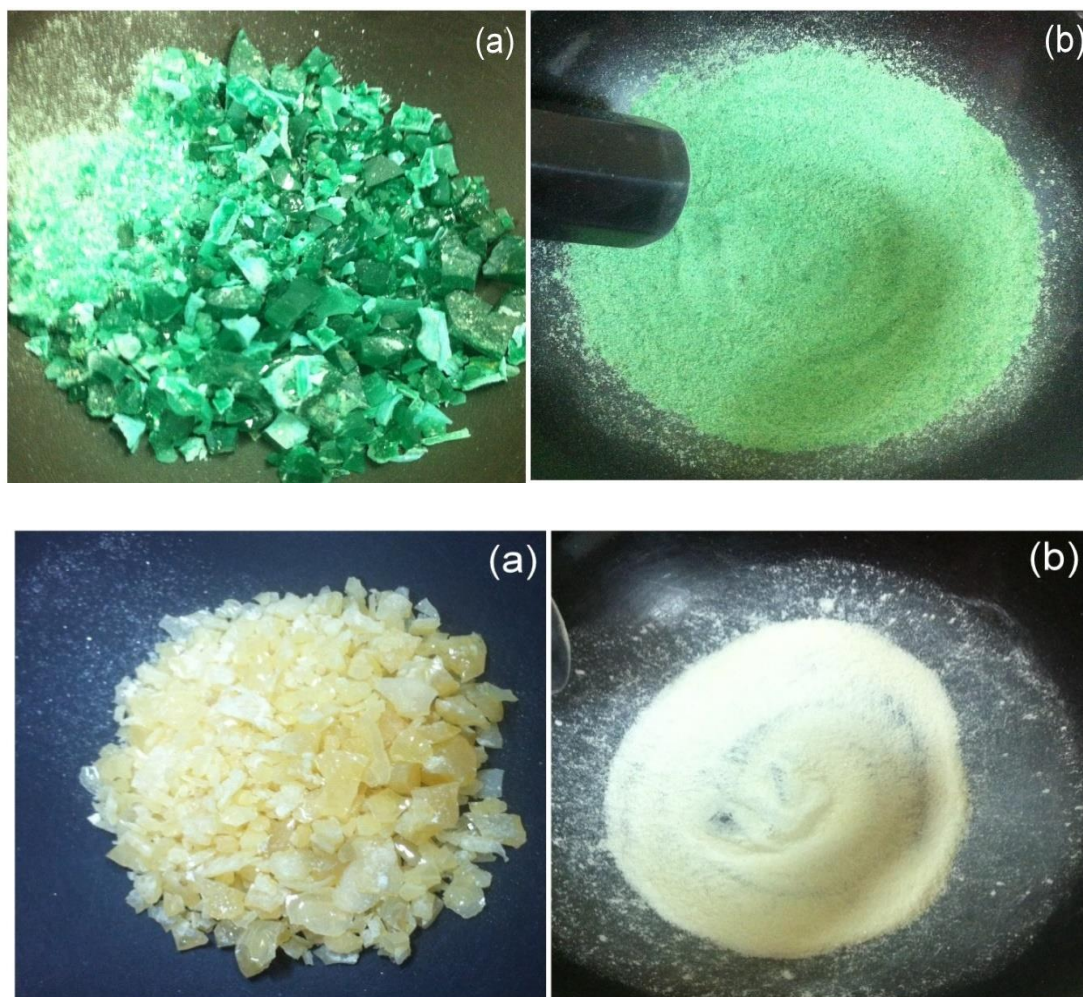
Figure 3.2.1. a) Cu doped before b) after grinding, 2. a) Se doped before b) after grinding
