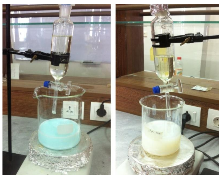
Figure 3.1. Stirring of Cu and Se doped TiO 2 .
