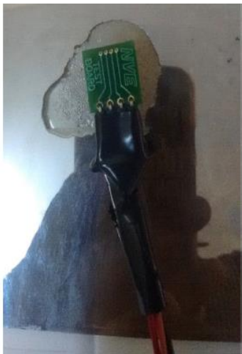
Figure 18: Spin tropic GMR sensor
