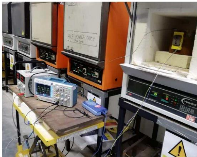
Figure 10: Actual setup using GMR sensor
