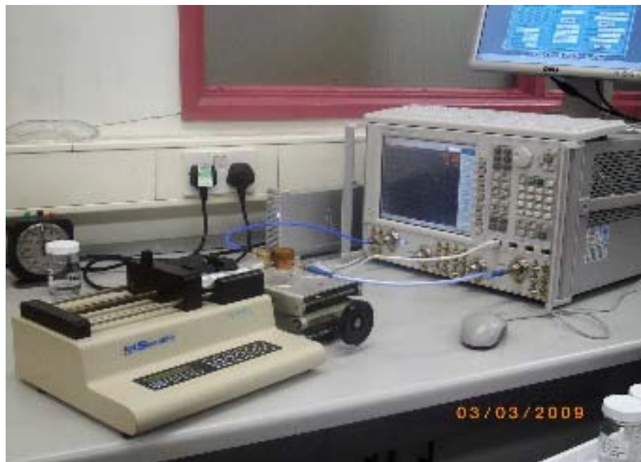
Figure 6.17. Photograph showing layout for conducting compositional analysis experiments in the miniaturised SDR based microfluidic device. The resonator is positioned on stand next to the syringe pump and the PNA is on the far right.
