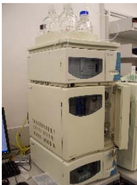
Figure 5.16. The Surveyor® LC pump is at the bottom of stack; the solvent containing vessels are on top.
