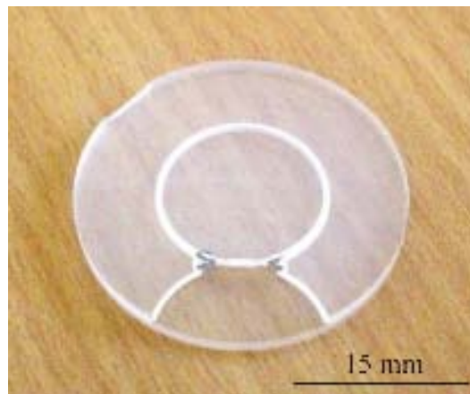
Figure 5.11. Laser machined channel in the region of high electric field on Teflon ® AF disc.
