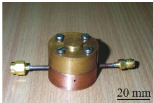
Figure 6.6. Photograph of the miniaturised SDR with the lid in upside down position.
