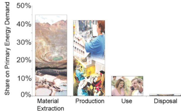
Figure 3.5 Primary Energy Demand of EEE along the product life cycle Source: Seliger et.al. (2008) Approaches to sustainable manufacturing, Int. J. Sustainable Manufacturing, Vol. 1, Nos. 1/2, pp. 58–77
