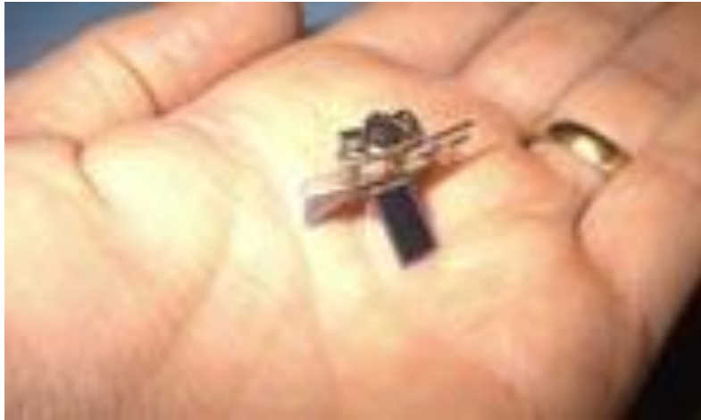
Figure 3: Micro Mechanical Flying Insect [6]
