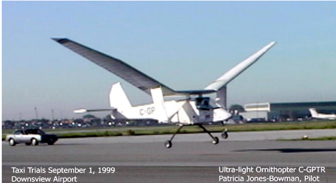
Figure 1: Harris/DeLaurier Model of Engine-Powered Piloted Ornithopter [3]
