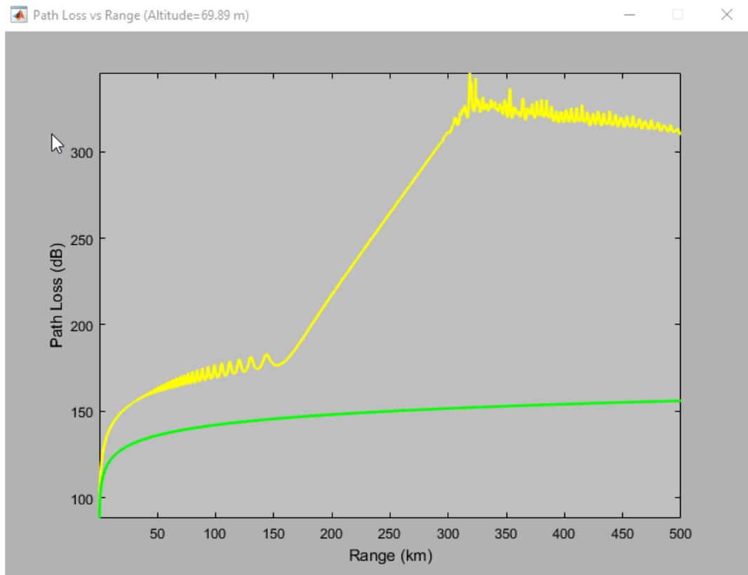
Figure 24 : Standard Condition Path Loss & FSPL Vs Range
