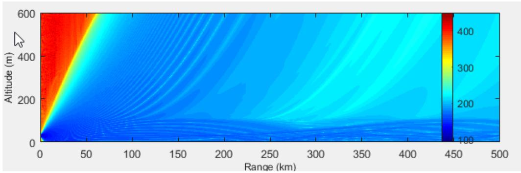
Figure 21 Path loss with Ducting Conditions
