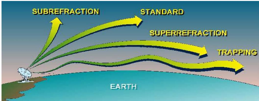
Figure 9 : Conditions of Refraction
