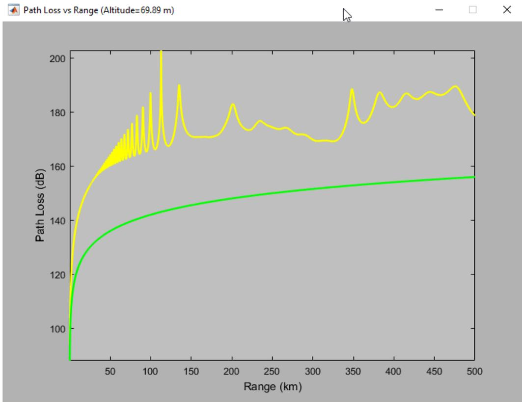
Figure 25: Ducting condition Path Loss Vs FSPL
