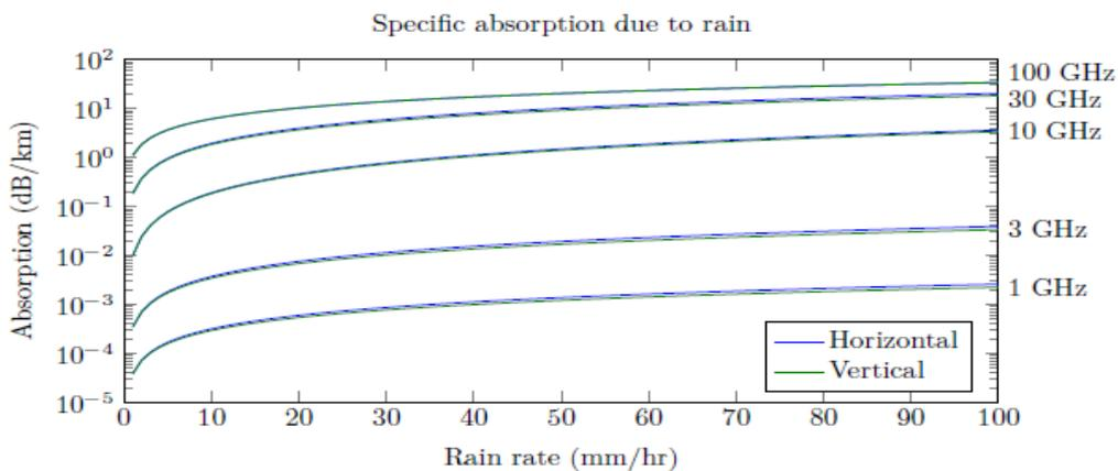
Figure 4: Graph Rain Vs Frequency
