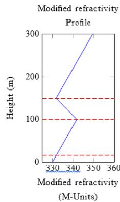
Figure 12 : Evaporation Duct
