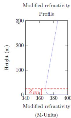
Figure 10 : Evaporation Duct
