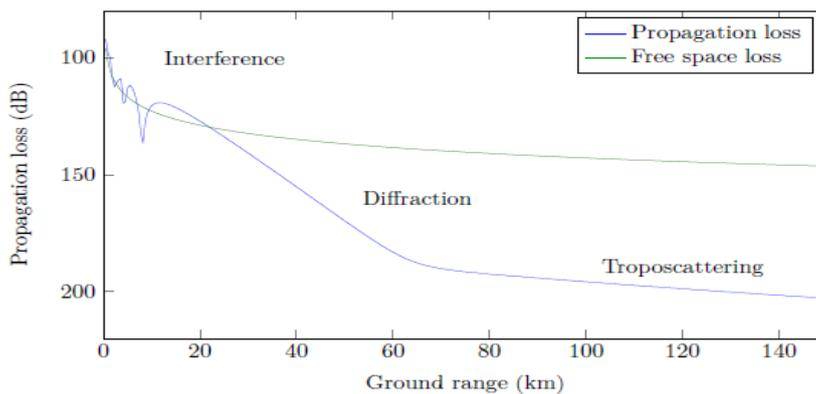
Figure 5 : Graph Range Vs Propagation loss
