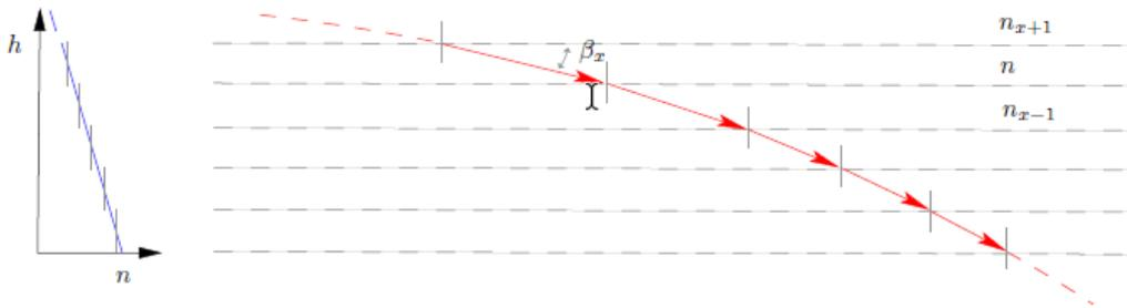
Figure 8 : Rays Propagation in Normal Atmosphere
