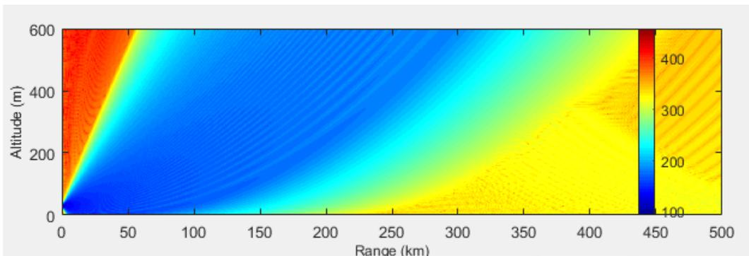
Figure 20 : Path loss with Standard Atmospheric Conditions
