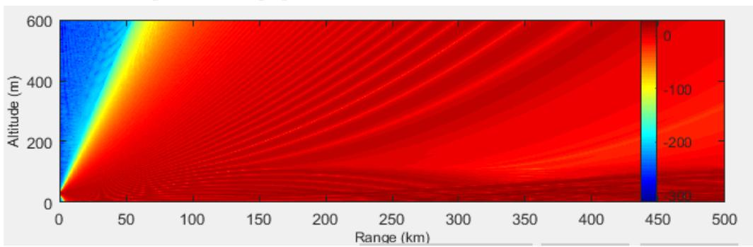
Figure 23: Propagation Factor with Surface Ducting Conditions
