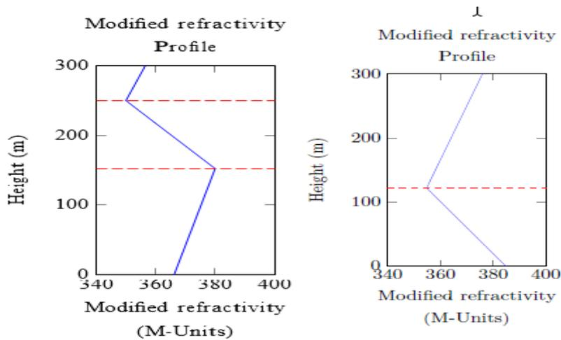
Figure 11 : Surface & Surface based Ducts
