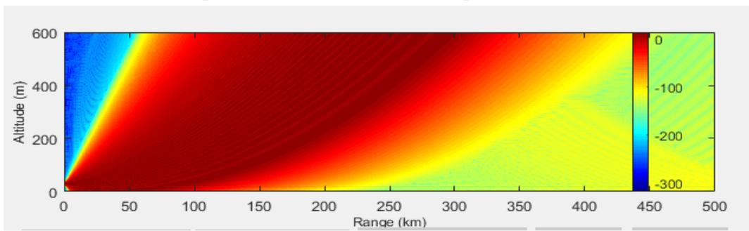
Figure 22: Propagation Factor with Standard Conditions
