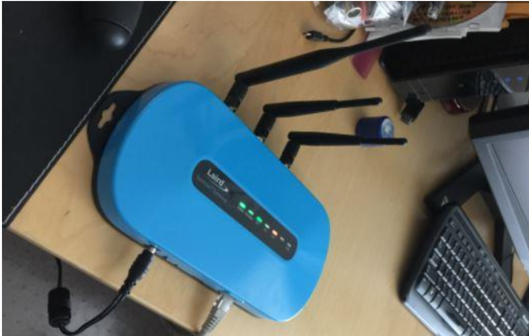
Fig 4.3. LoRa Gateway used in testing
