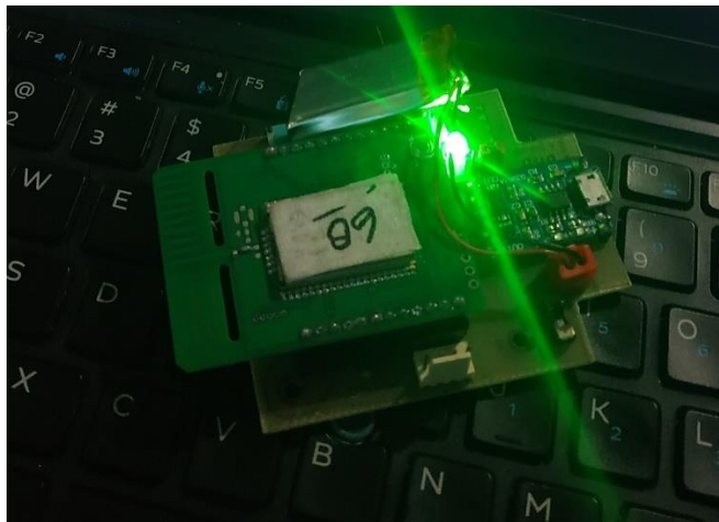
Fig 4.2. End node during testing
