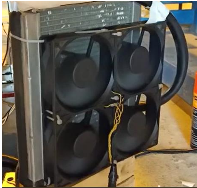
Figure 7. Heat Rejection System
