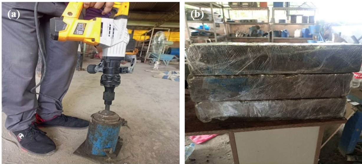
Figure 3.4.3 (a) Casting of RCCP cylinders.
