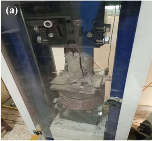
Figure 3.4.4 (a) RCCP compression test.
