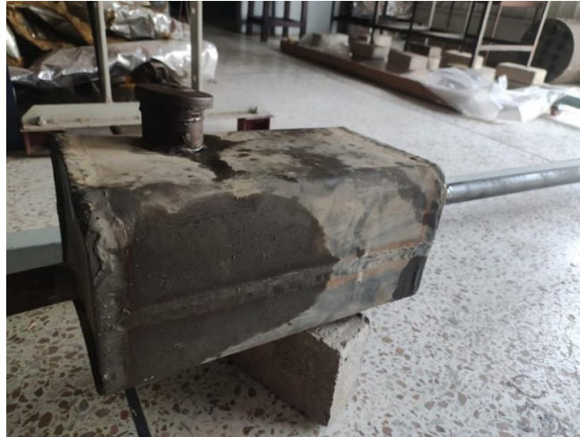
Figure 32: Oil Reservoir for pump
