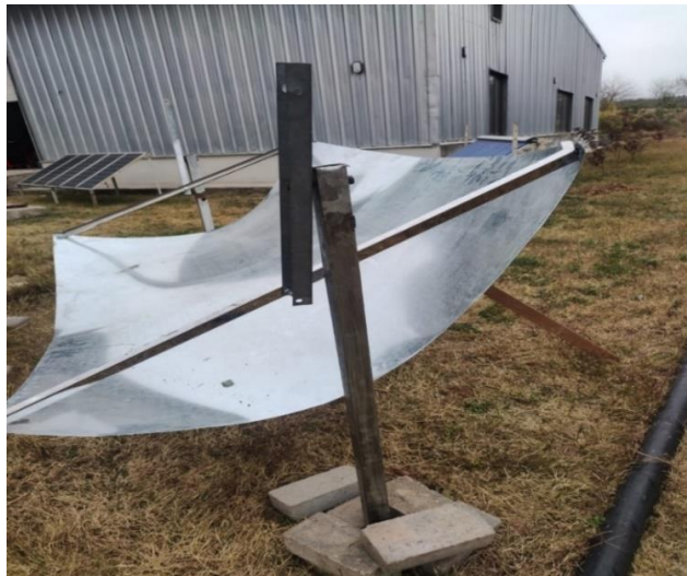
Figure 27: Assembling of Solar Collector
