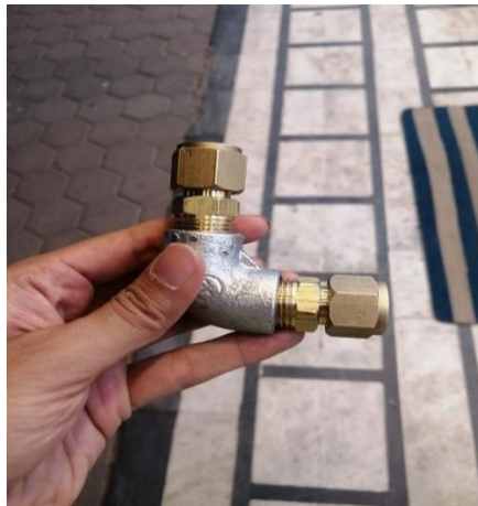
Figure 31: Flaring Nipple assembly for copper tubes
