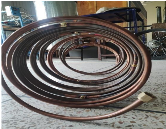
Figure 30: Spiral copper tubes for helical coil heat exchanger
