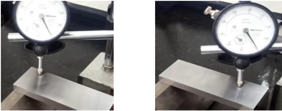
Fig 5.5 shows flatness test on workpiece
