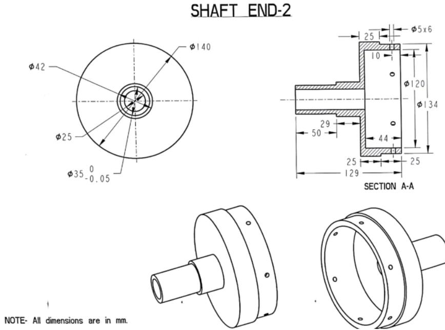
**Figure 19: Engineering Drawings of Shaft Ends**
