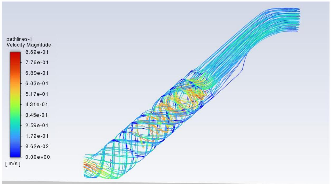
**Figure 14: Path lines depicting the velocity and direction of water surrounding the screw**
