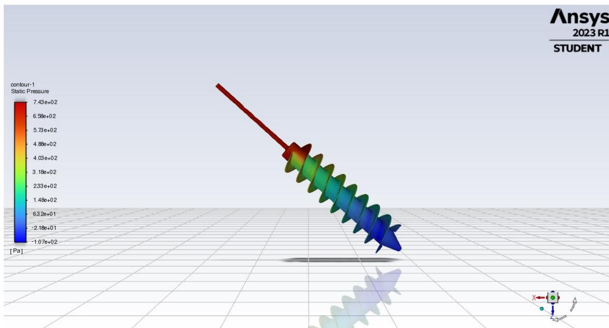
**Figure 15: Static Pressure Contours at Different Locations around the Screw**
