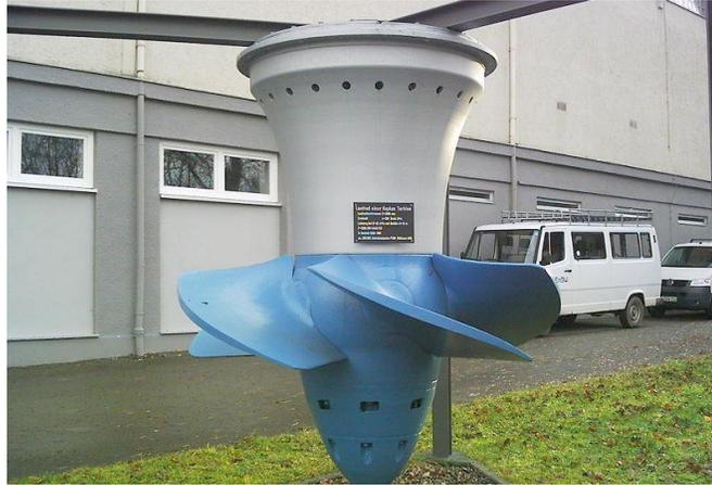
**Figure 3: Real Life Model of Kaplan Turbine**
