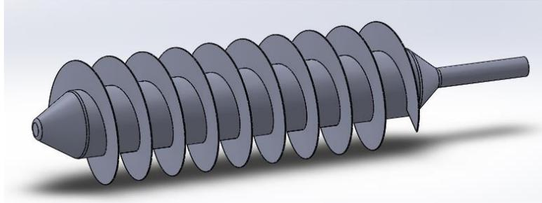
**Figure 8: CAD model of Screw Runner**
