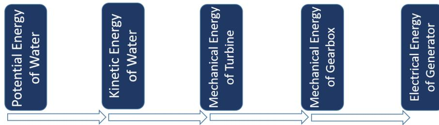
**Figure 6: Working Principle of an Archimedean Turbine**
