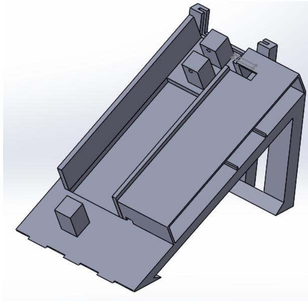
**Figure 10: CAD Model of the Turbine Frame**
