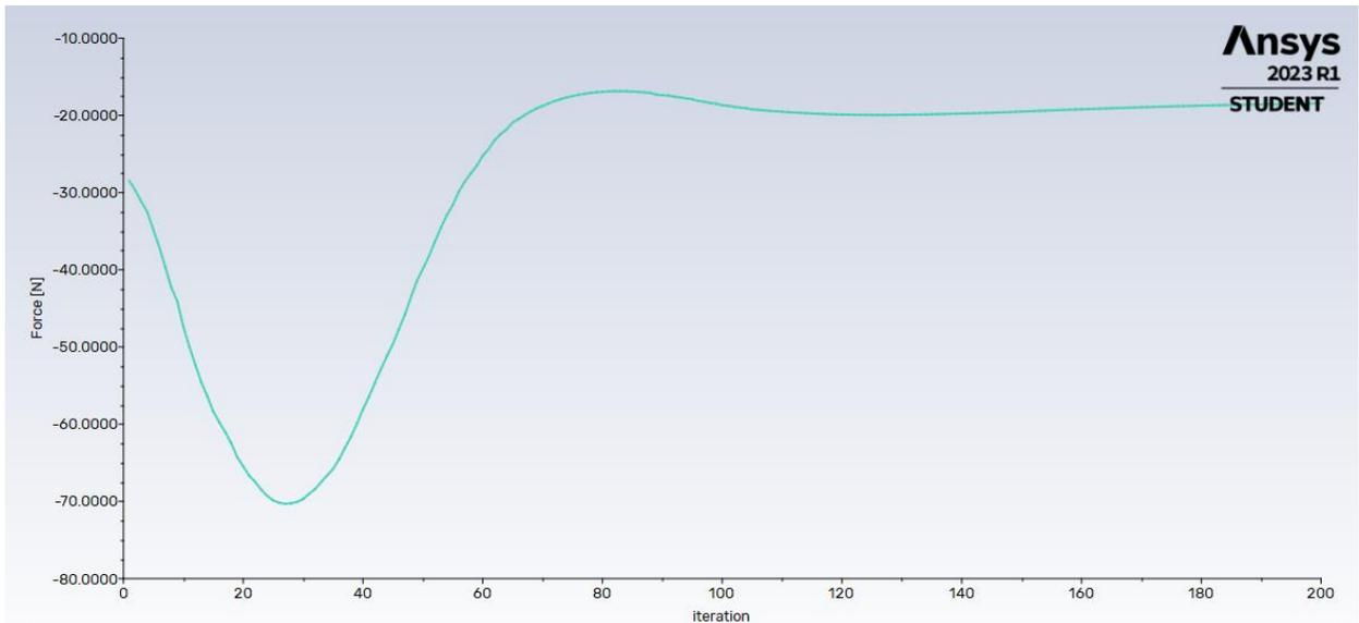
**Figure 16: Graph Showing Hydrodynamic Force Convergence of Designed Model**
