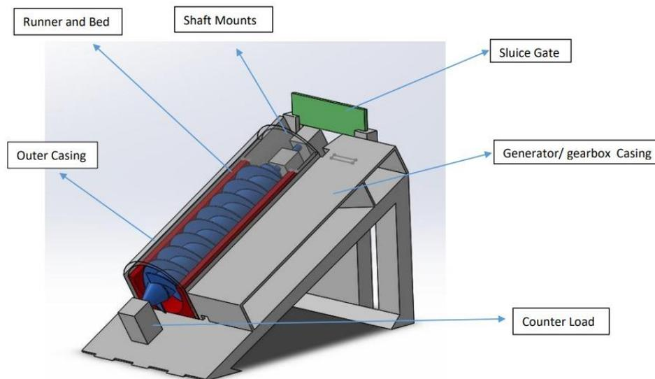
**Figure 7: Main Components of an Archimedean Turbine**
