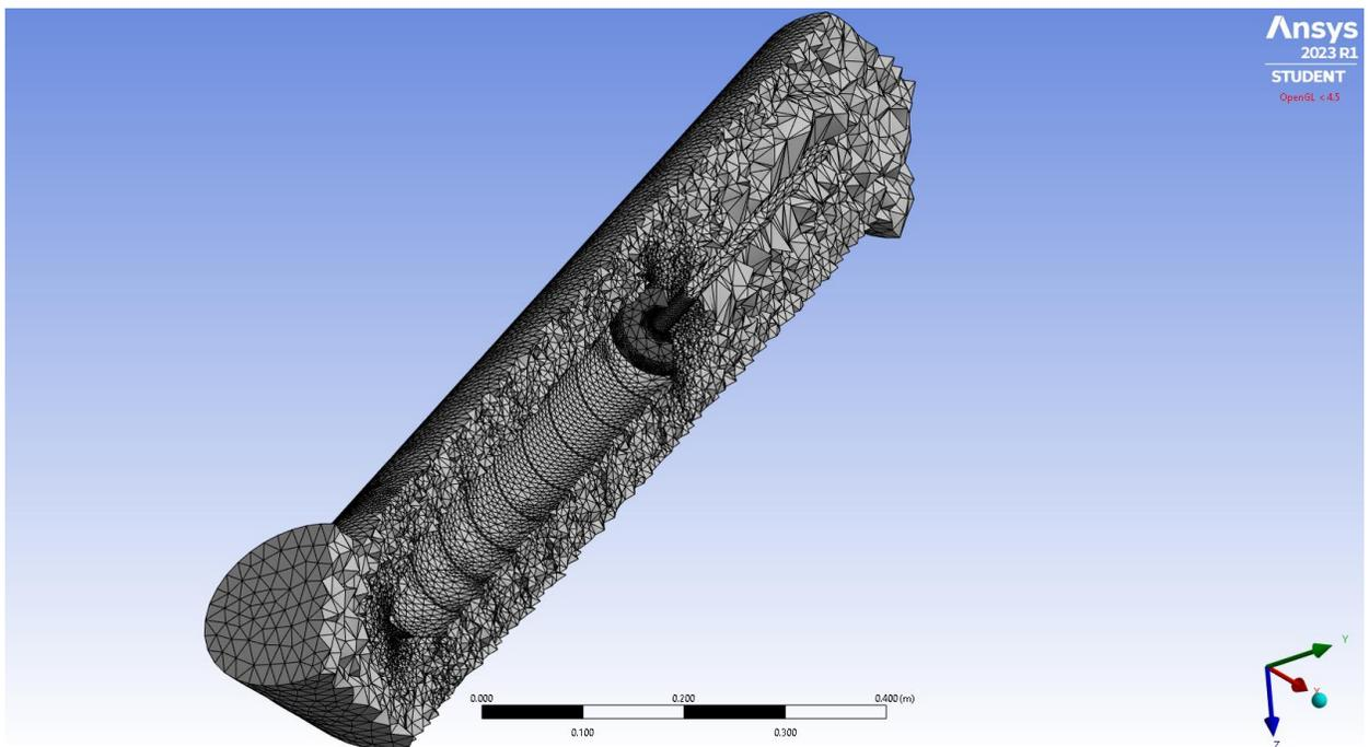
**Figure 12: Mesh Generation for CFD Analysis**
