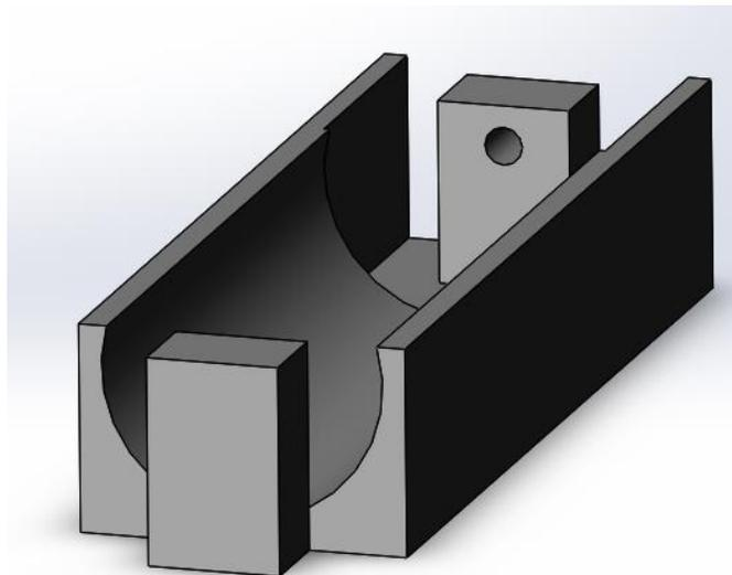
**Figure 9: CAD Model of the Trough of the Turbine**
