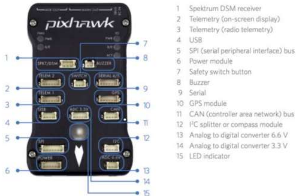
Figure 22 Autopilot with Interface Details
