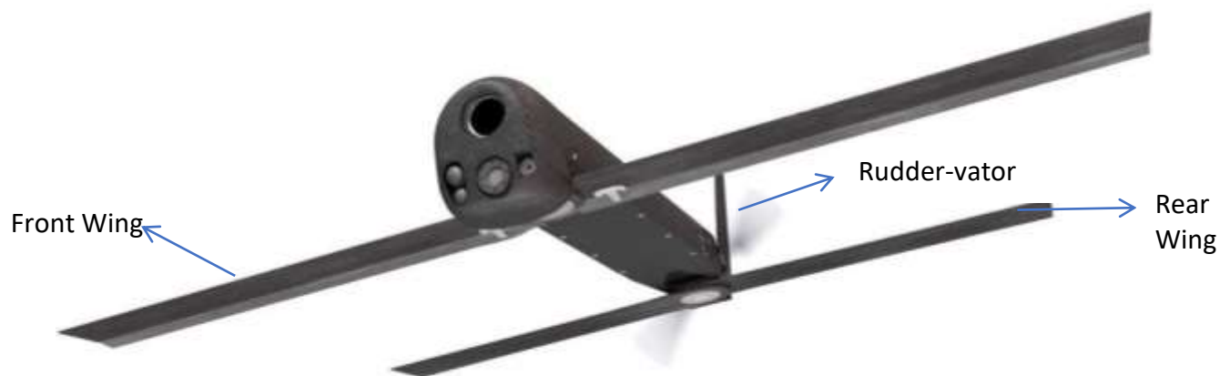
Figure 3 Control Surfaces: Loitering Munition UAV [13]
