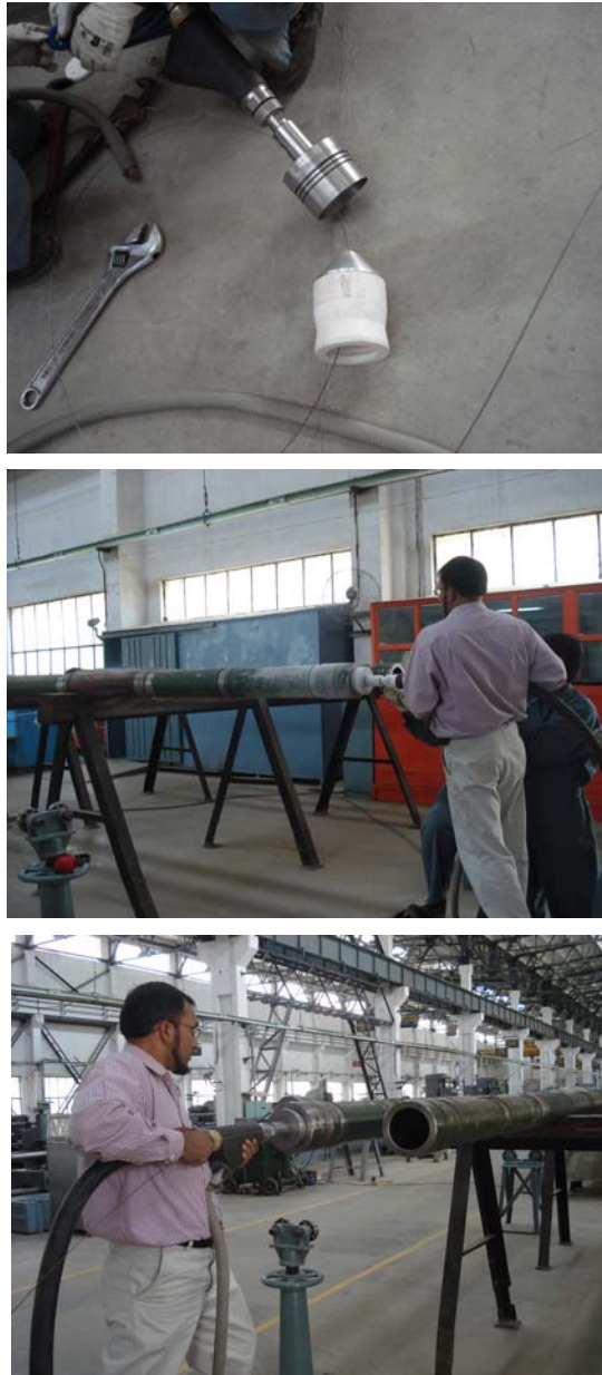
Figure-5.6:- Barrel Cleaning in Process
