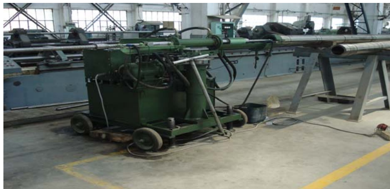
Figure- 2.10: – Bore Cleaning at HIT
