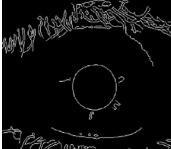
Figure 7.2: sobel edge detected image of the eye
