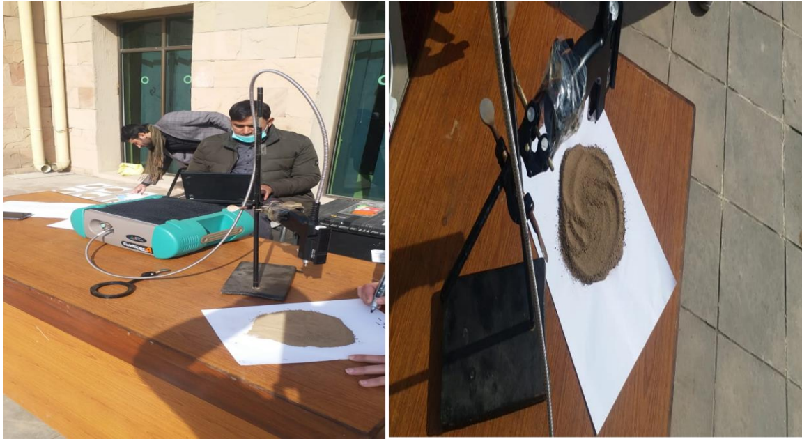
Figure 2.8. (a) and (b) Spectral Signature of Soil using ASD FiledSpec.
