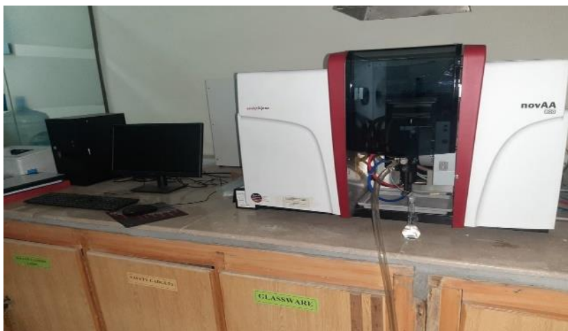
Figure 9: Atomic Absorption Spectrophotometer (AAS) of wastewater laboratory IESE, NUST
