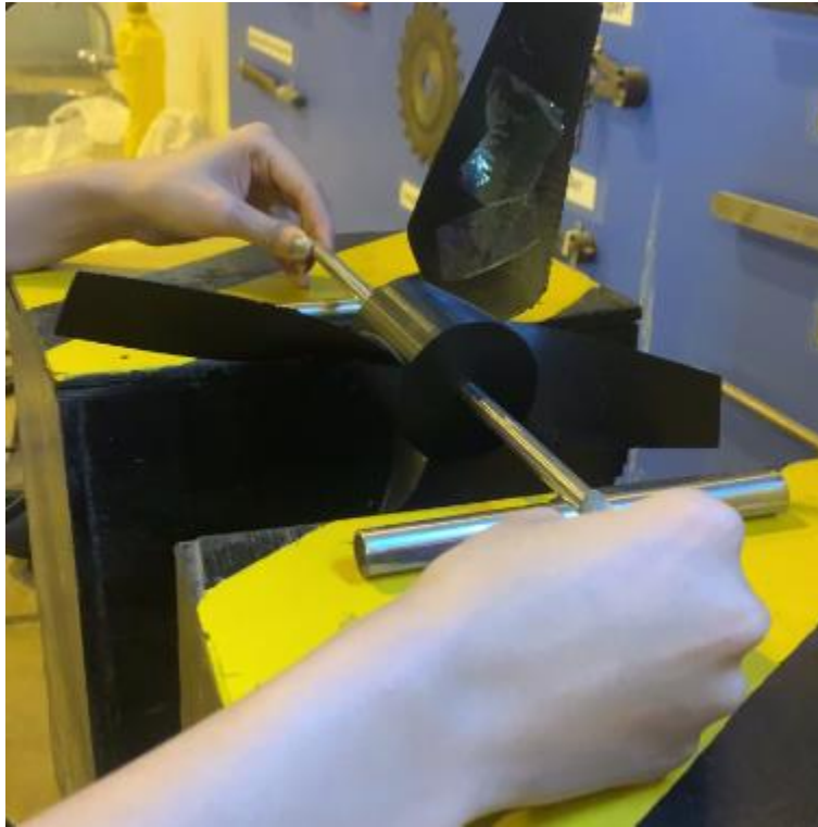
Figure 27: Balancing of fan
