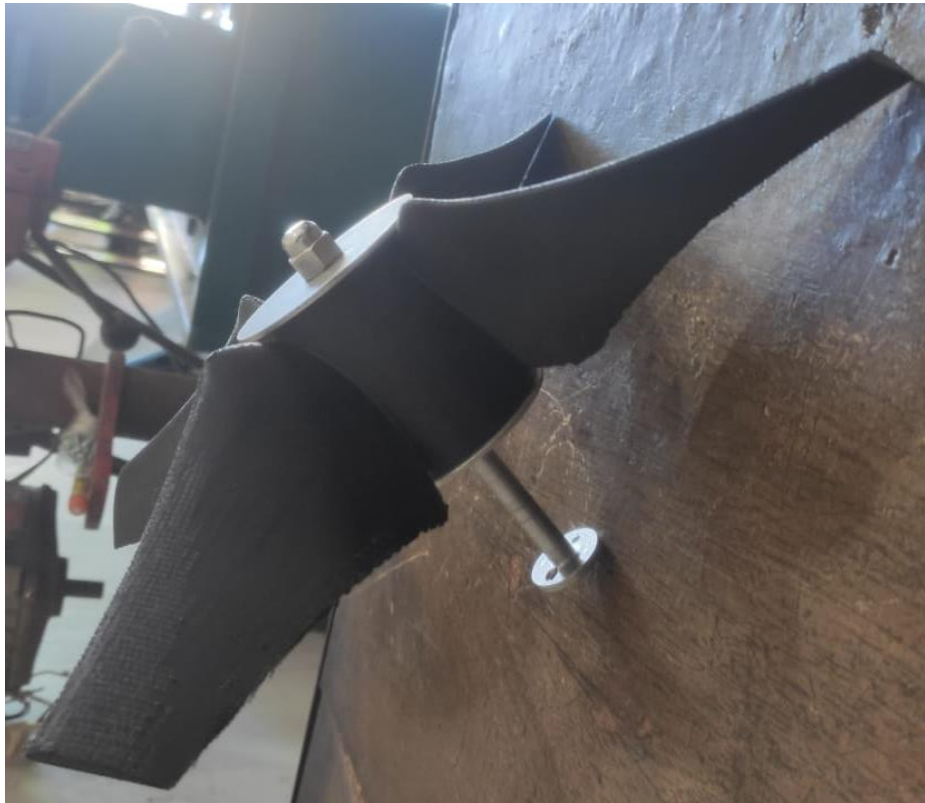
Figure 26: Flanges and shaft
