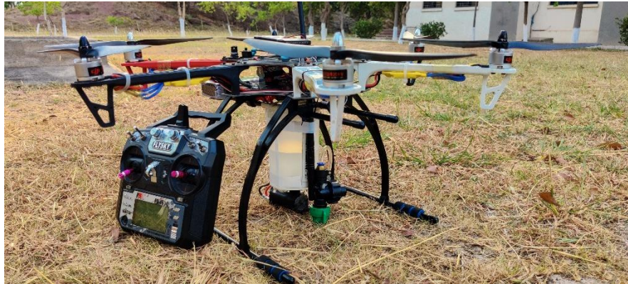
Figure 12 UAV with sprayer tank and Nozzle
