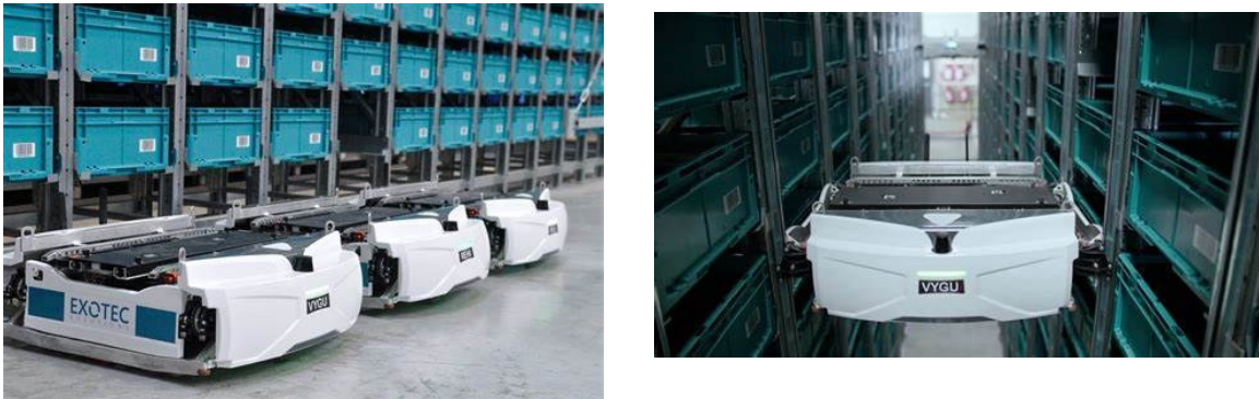
Figure 1 Exotec Skypod warehouse robot
