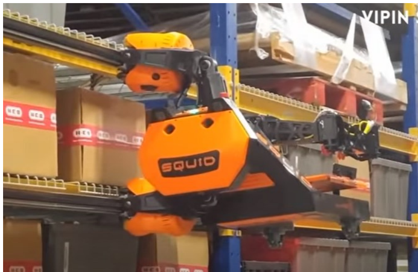
Figure 2 SquidBot rack climbing robot
