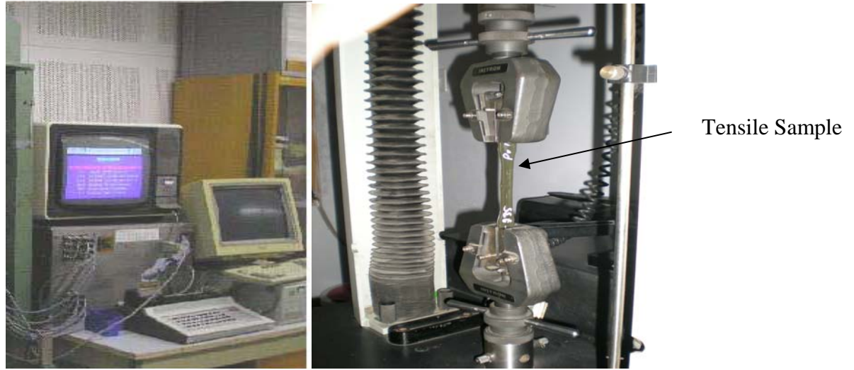
FIG 5.21 INSTRON UNIVERSAL TESTING 10 KN MACHINE
