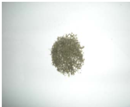
Figure 5.8 Grain shaped test sample for TGA
