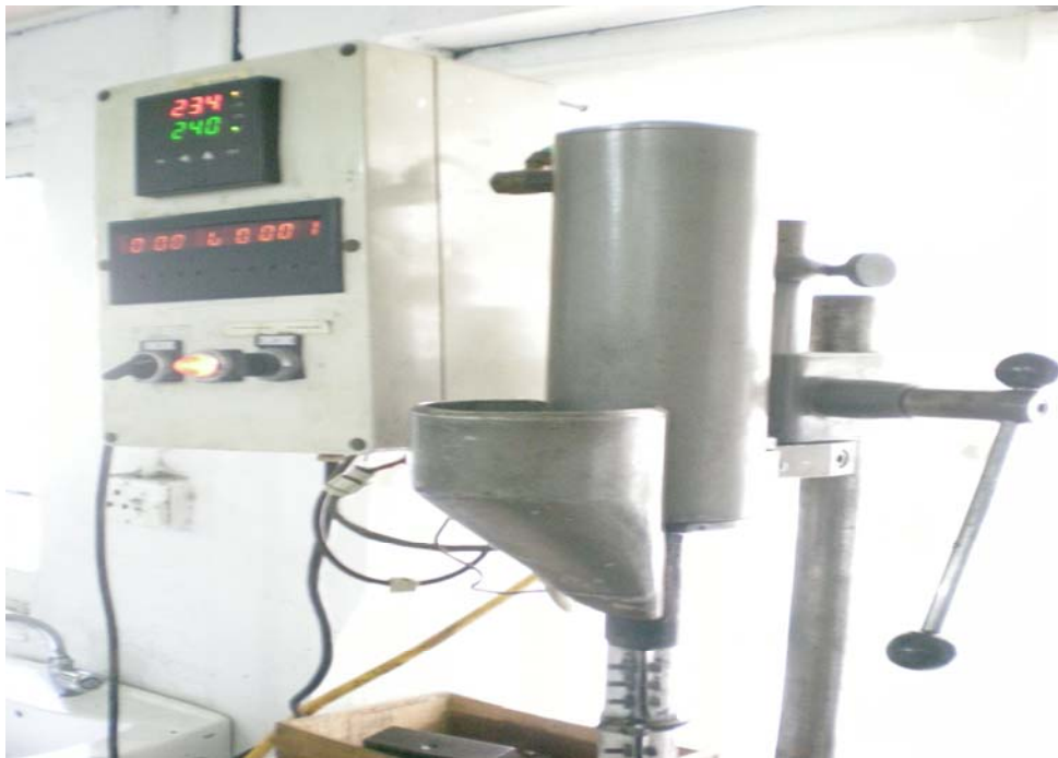
Fig 5.20 RN 350 injection molding machine
