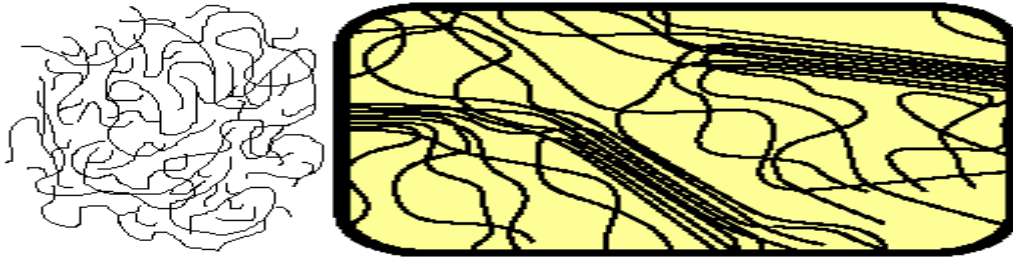
Figure 2.13, Amorphous Polymers structure[39]
