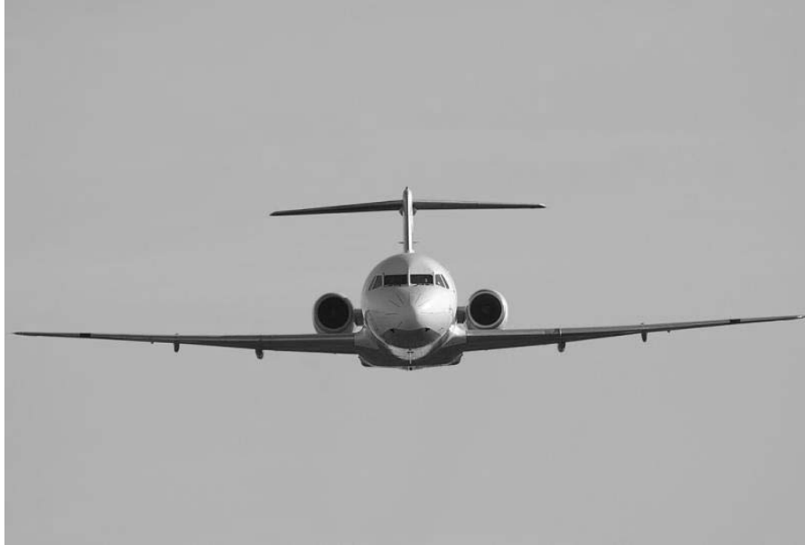
Figure 1.2: T-Tail configuration in Fokker 100 aircraft
