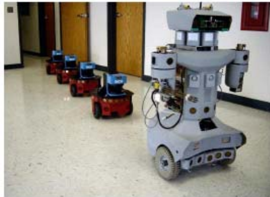
Figure1.4. A ‘Leader’ robot coordinates by communicating with the follower robots
