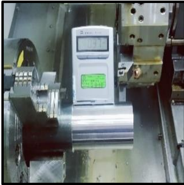
Figure 3.3; Pictorial view of TR 110 Roughness meter
