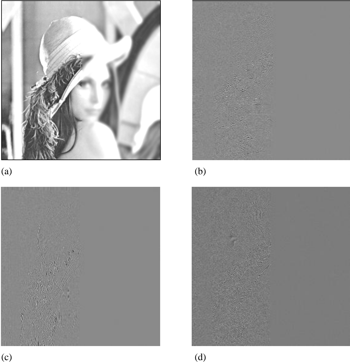
Figure 5.4: Wavelet coefficients of left-focused Lena image (a) Approximate, (b) Horizontal, (c) Vertical and (d) Diagonal
