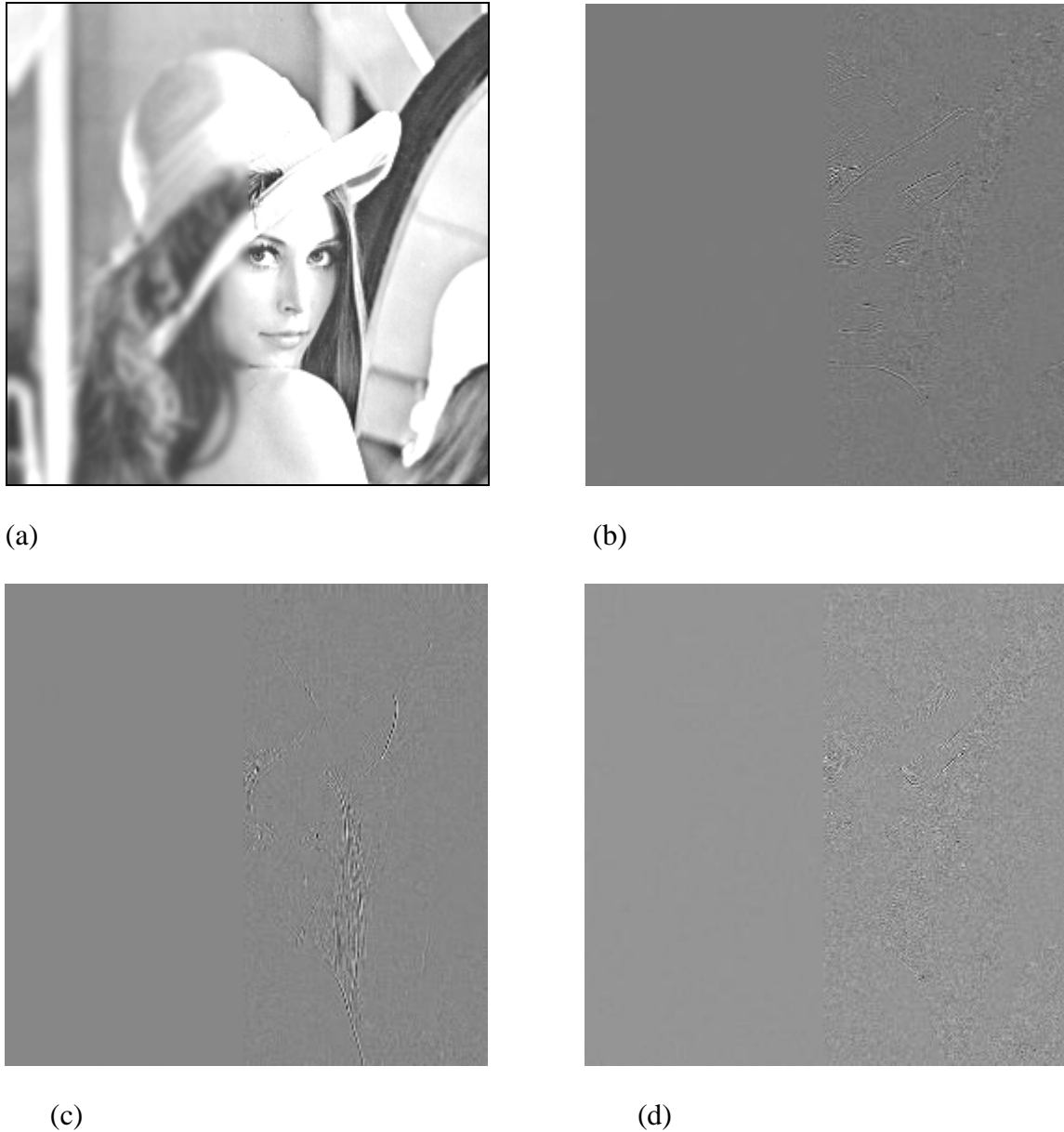
Figure 5.5: Wavelet coefficients of right-focused Lena image (a) Approximate, (b) Horizontal, (c) Vertical and (d) Diagonal
