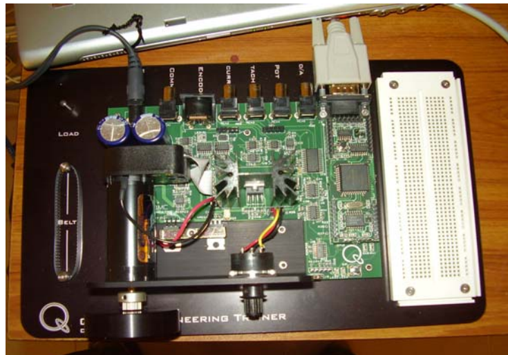
Figure 5. 27: Experimental setup with the QET DC Motor Kit from Quanser.
