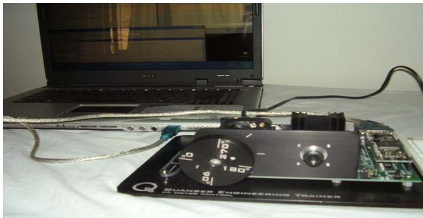
Figure 3.45: Quanser's DC motor kit used to test the approach.
