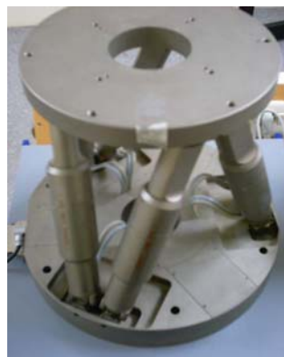
Figure 2.26: Six degree of freedom Hexapod by PI.
