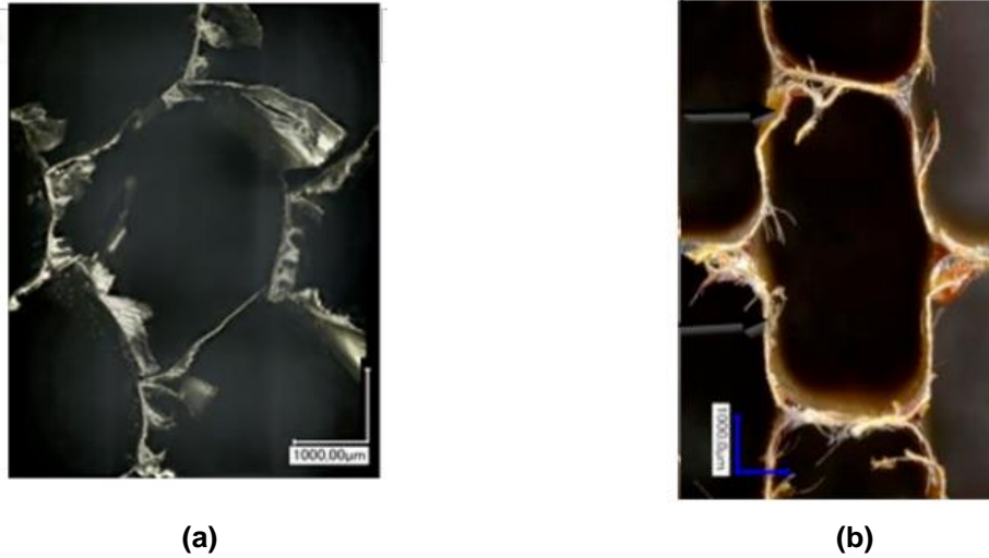
Figure 6 (a) Burr Formation (Jaafar, Makich, et al., 2021) (b) Delamination and tearing of wall (Zarrouk, Salhi, Nouari, et al., 2021)
