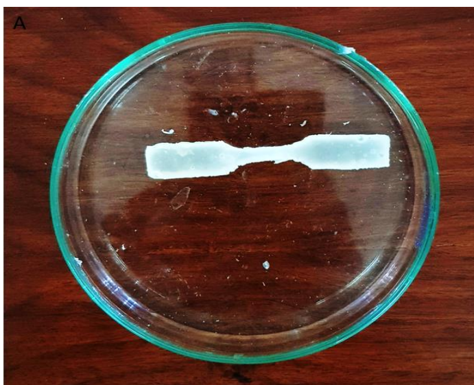
Figure 17: Dumbbell shape sample prepared for tensile testing
