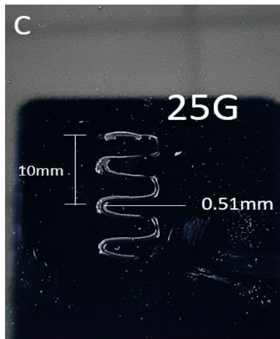
Figure 10: Printed single layer using 25G needle and analyzed through ImageJ software
