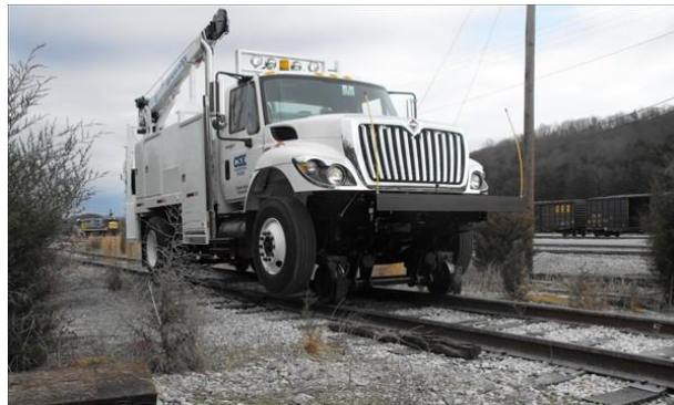
Figure 4: A Hi-Rail Truck Operating on Railway Tracks
