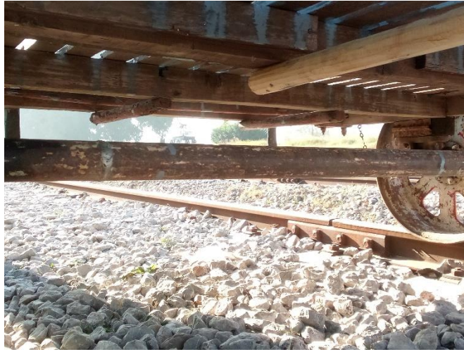
Figure 22: Wheelset view from below the chassis
