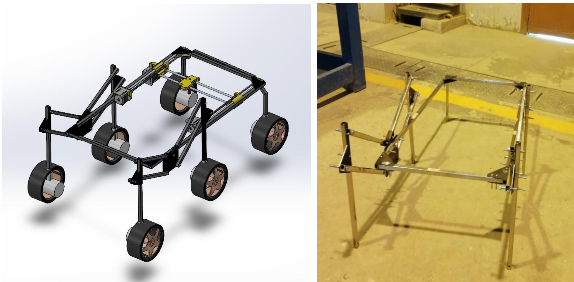
Figure 32 Comparison of Robot Design Model and Fabricated Frame
