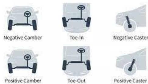
Figure 2: Camber, Castor and Toe Angle
