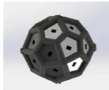
Figure 10 Camera Enclosure for 24 cameras
