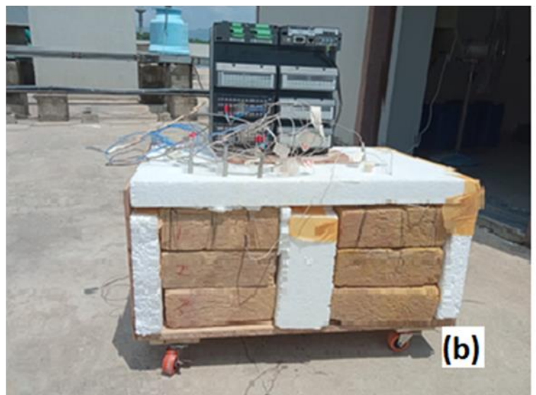
Figure 7. Testing of Brick Walls (a) With lamp Heat Source, (b) With Sunlight in Open Environment
