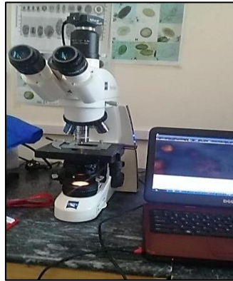
Figure 3.4: Assembly of optical microscope, IDS-digital camera and computer system
