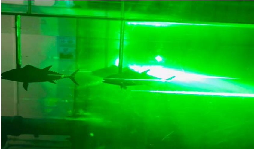
Figure 23 Fish Testing PIV
