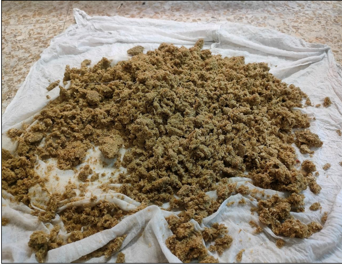
(b) TiO 2 Pretreated WS after washing
