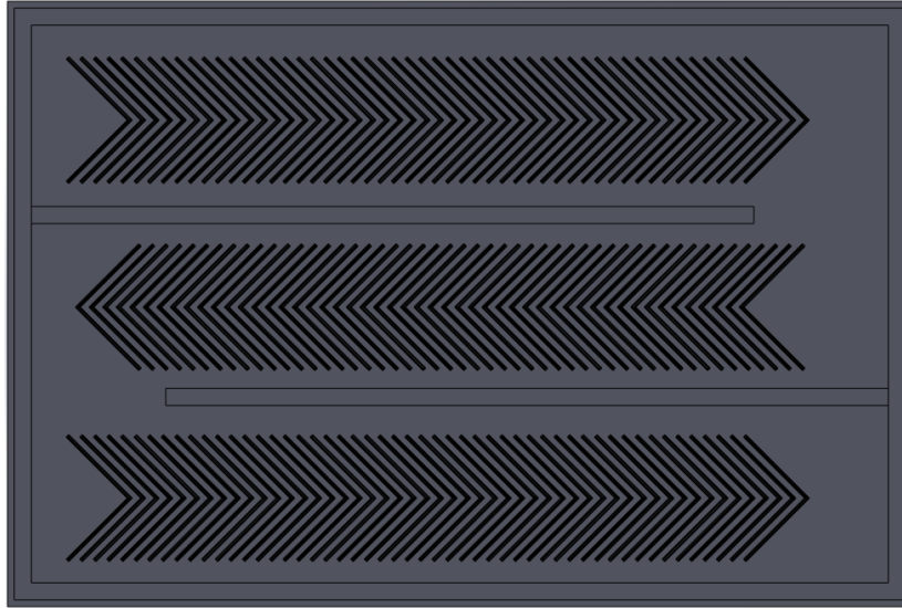
Figure 4: Aluminum Sheet with V shaped pattern engrooved on it
