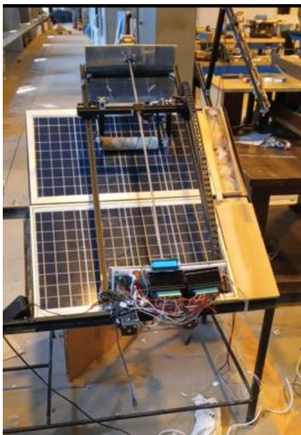
Figure 23: Smart Solar Panel Cooling and Cleaning system
