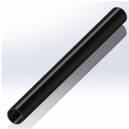
Figure 18 Figure shows link 3 made of carbon fiber
