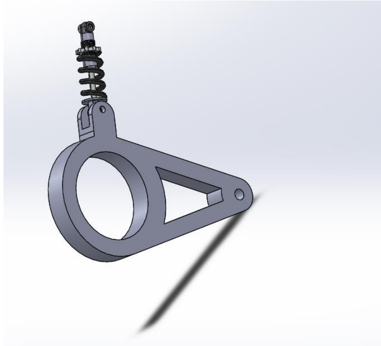
Figure 19: Rear Axle Mount
