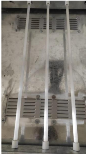
Figure 23. Shows the ceramic rods of heater on the inside of the body
