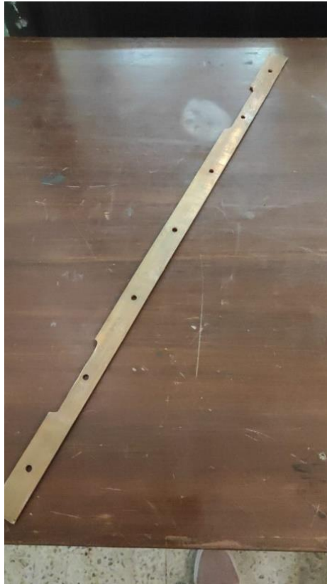
Figure 24. Shows the copper sheet which is used to connect the ceramic rods with the main power supply
