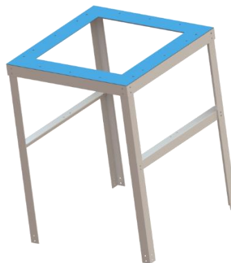
Figure 9. Shows the frame in solidworks.
