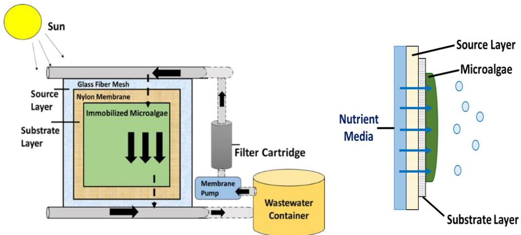
Figure 2. 4 Diagrammatic representation of porous substrate bioreactor (PSBR)
