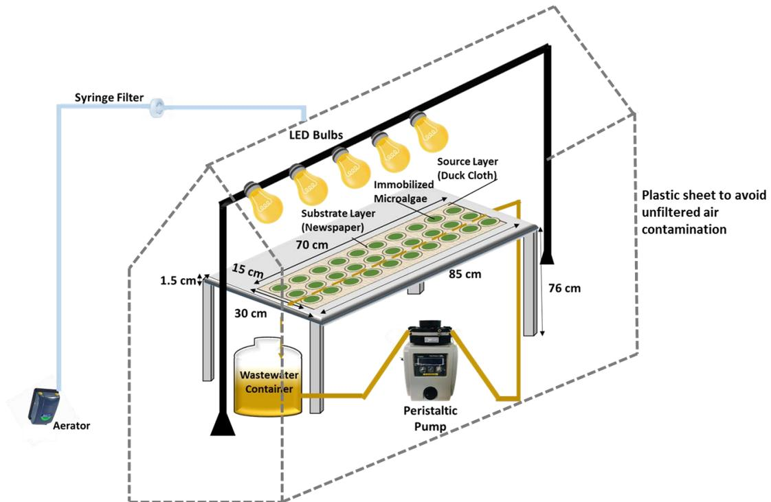
**Figure 3. 2 Diagrammatic representation of the laboratory scale twin layer cultivation system (TLS)**
