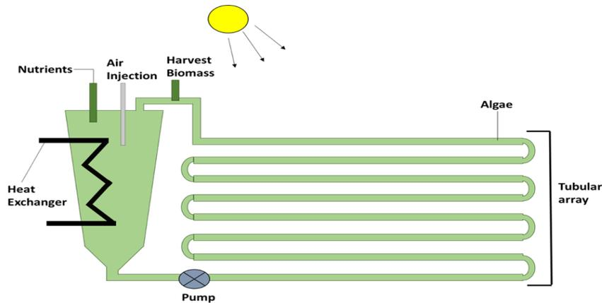
**Figure 2. 3 Diagrammatic representation of tubular photobioreactor**
