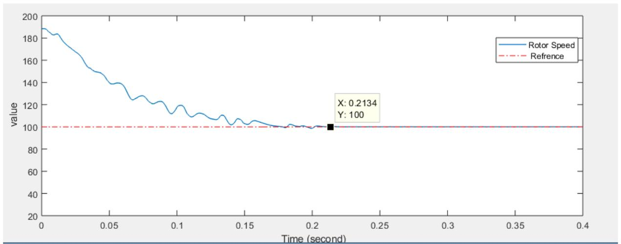
Figure 6.2: Speed control of motor
