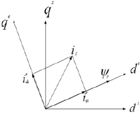
Figure 5.2: Decoupling between rotor flux and torque
