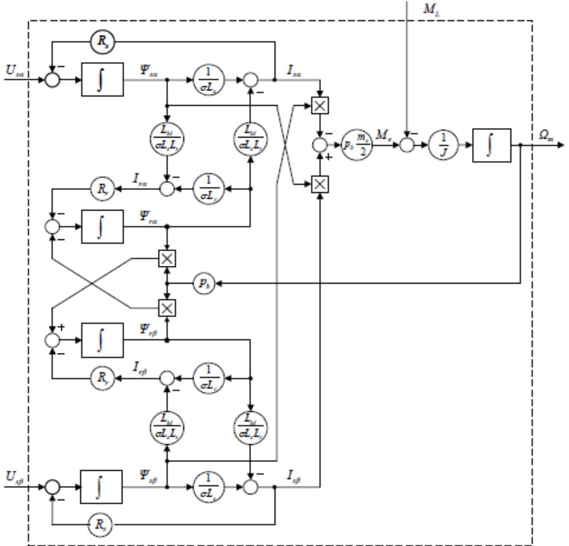
Figure 3.4: Induction motor block diagram representation in  $\alpha - \beta$  coordinates
