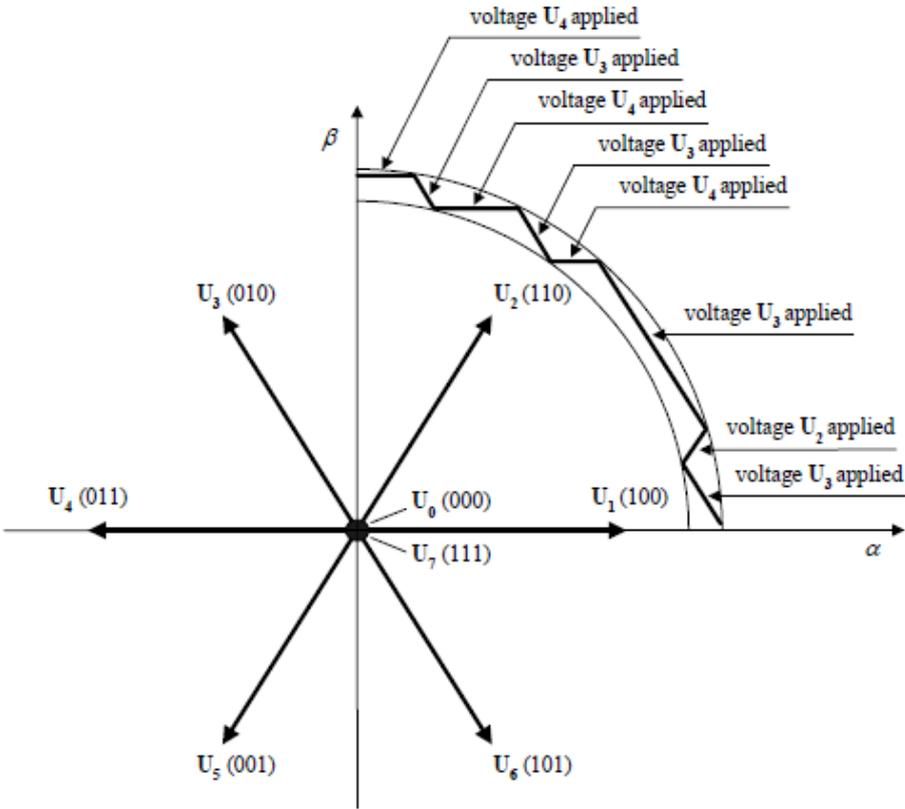
Figure 5.6: Stator flux trajectory formation by appropriate selection of voltage vectors
