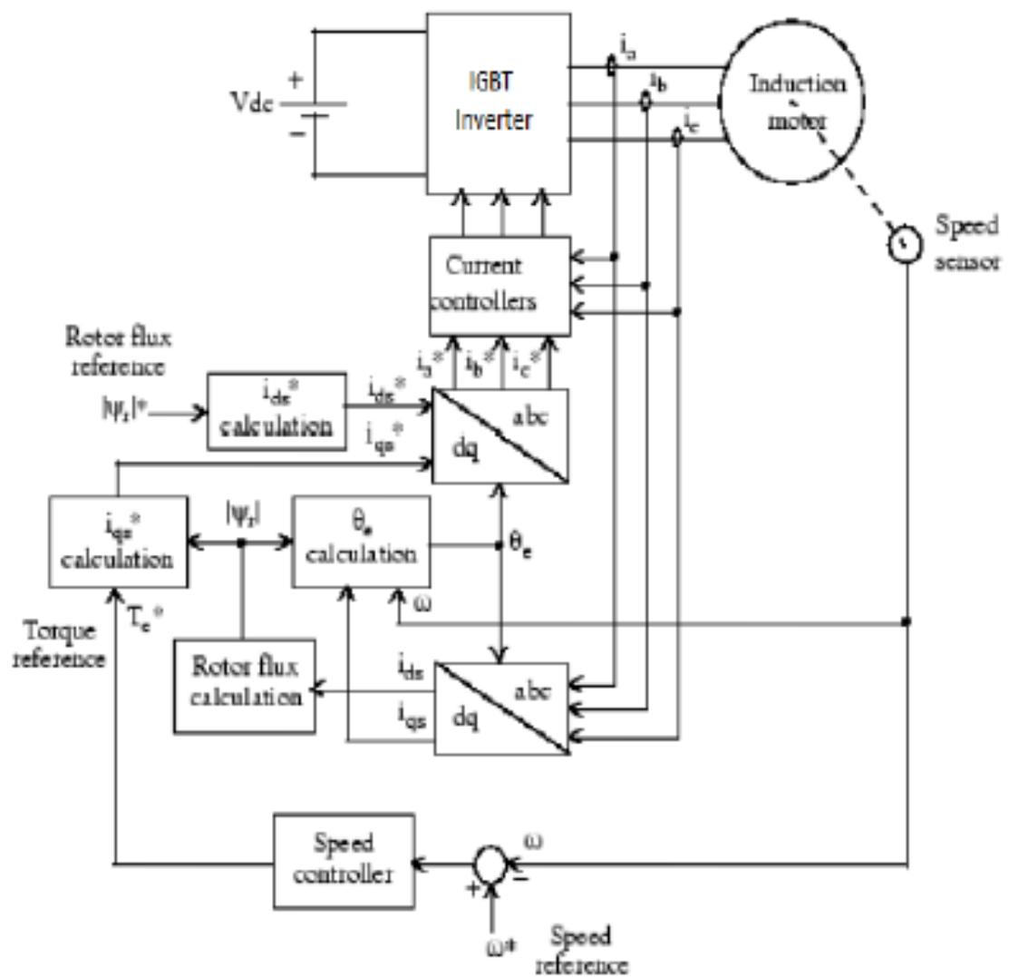
Figure 5.3: Block diagram representation of FOC [25]
