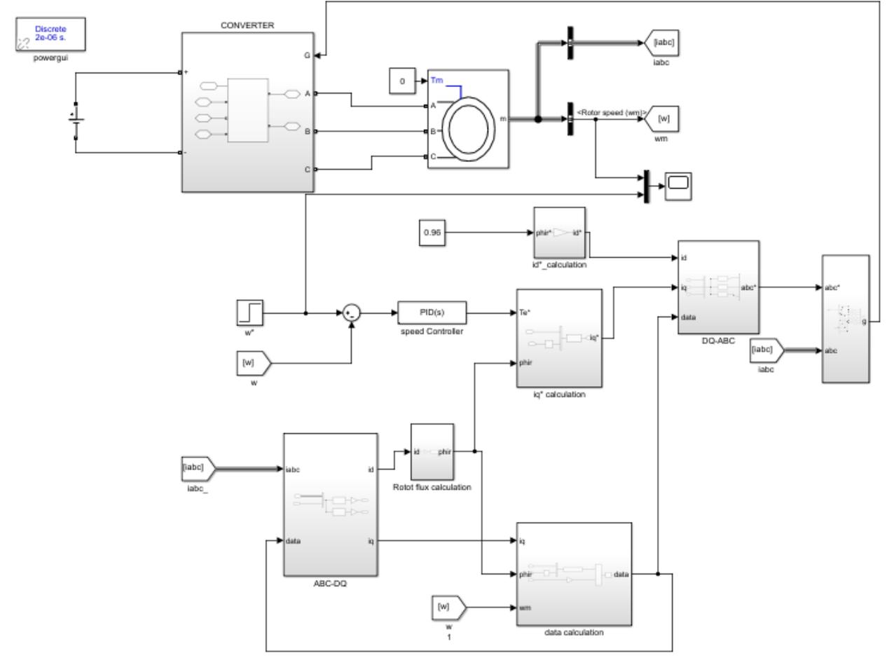
Figure 5.4: Simulink Diagram of FOC
