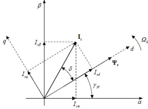
Figure 4.1: Induction motor's vector diagram in stationary ( $\alpha - \beta$ ) and rotating (d-q) coordinates
