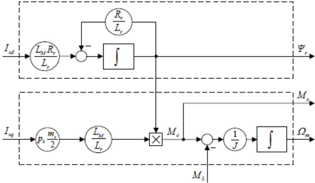
Figure 4.2: Induction motor block diagram in d-q coordinates
