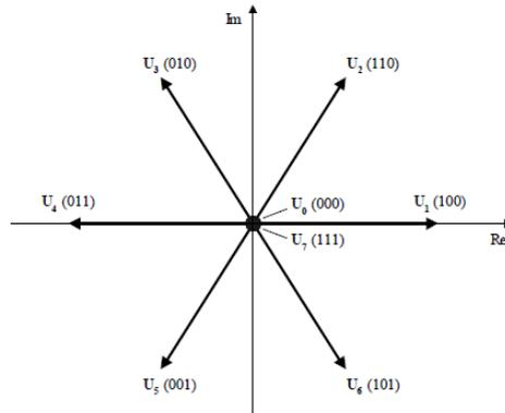
Figure 5.5: Space vectors representation of inverter output voltage
