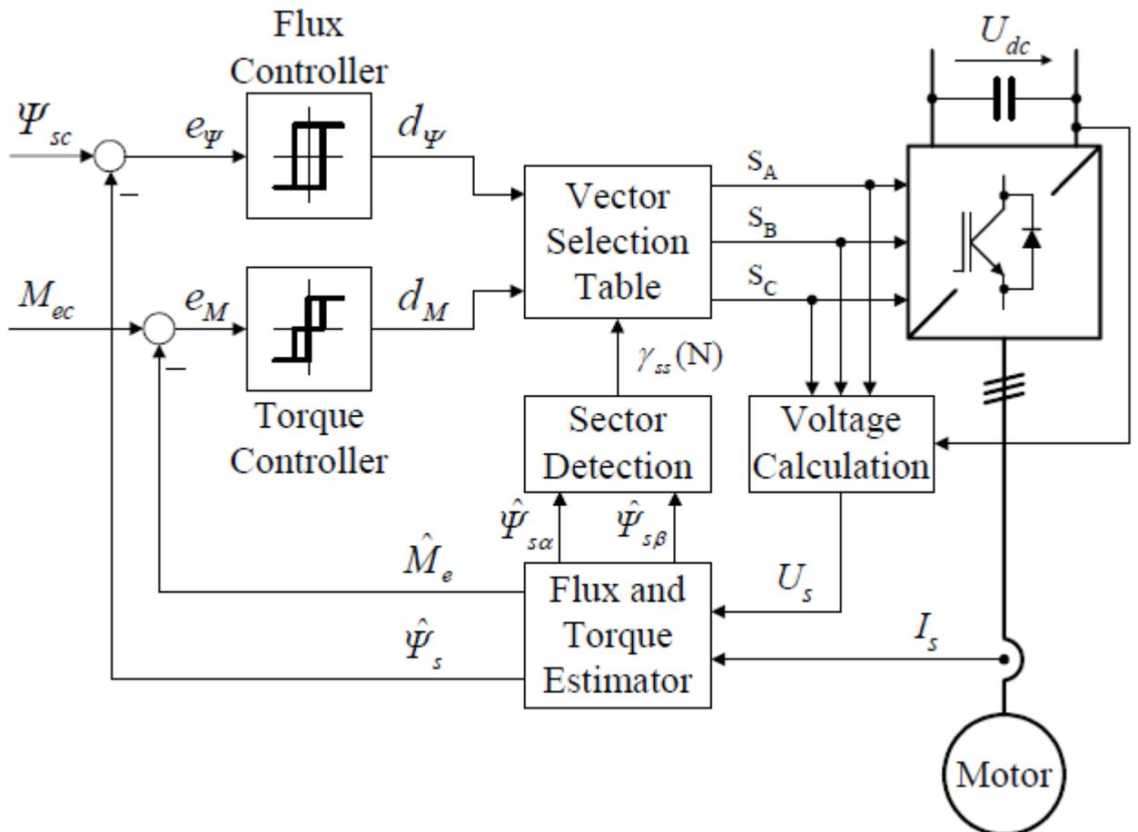
Figure 5.7: Block diagram of Direct torque control
