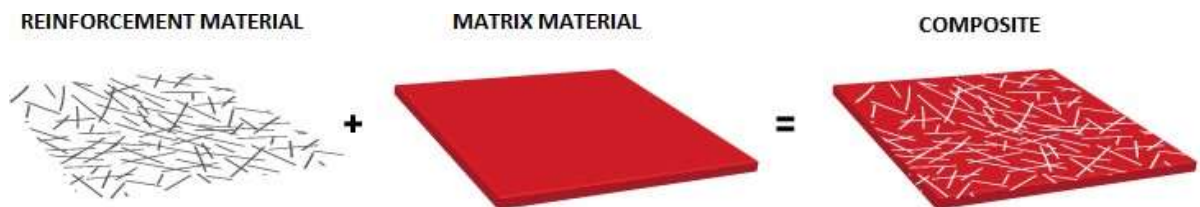
Figure 2 general structure of composites
