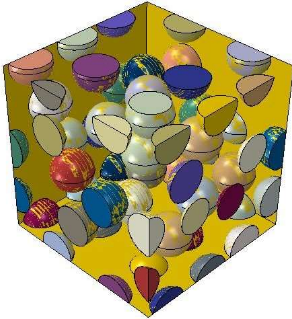
Figure 10 Epoxy-silica composite with 20% volume fraction of silica
