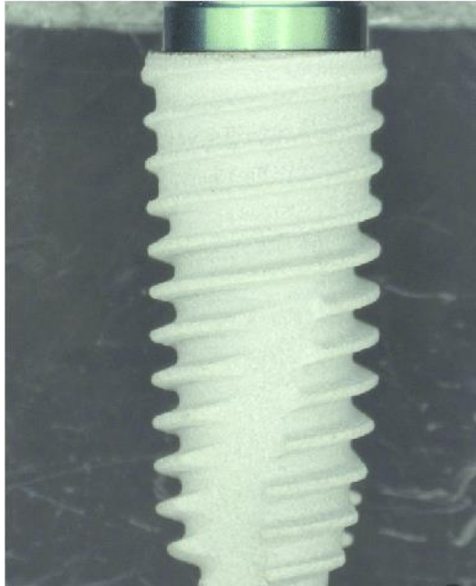
Figure 5 Hydroxyapatite coating on dental implant [14]
