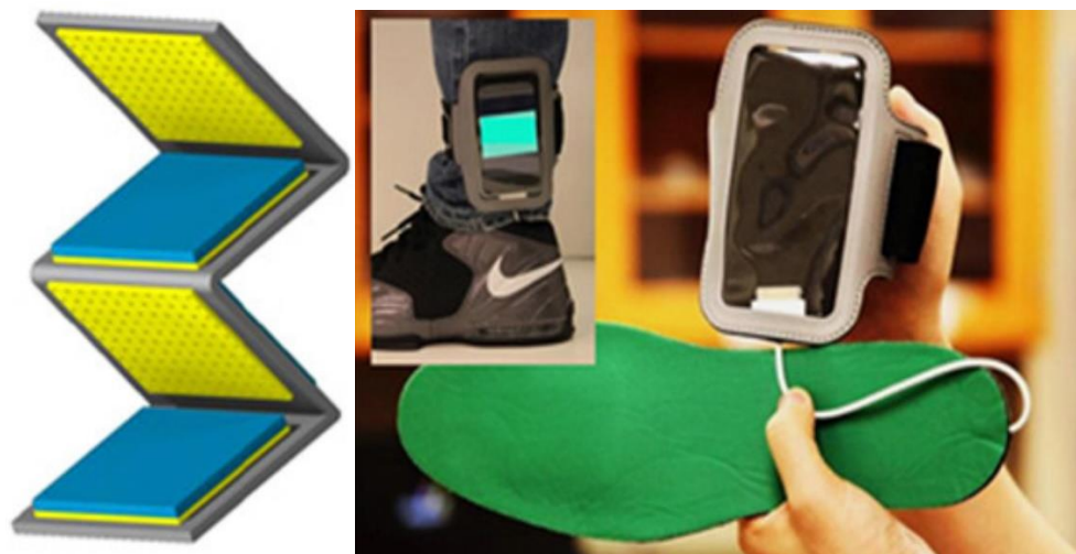
Fig 2. 2: a shoe insole TENG device with a folded structure that can light up LEDs on the application of pressure
