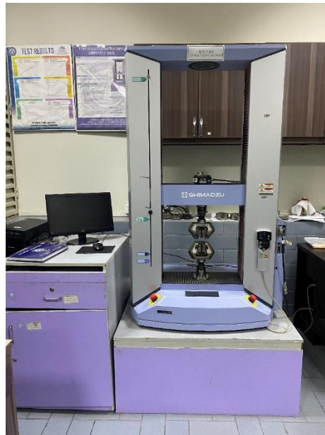
Figure 14. Universal testing machine at SCME NUST
