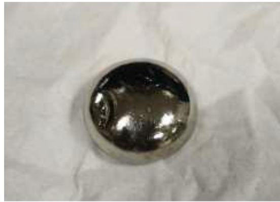
Figure 6. Solidified alloy button
