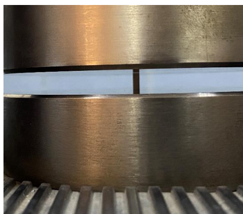
Figure 13. Alloy sample During compression testing
