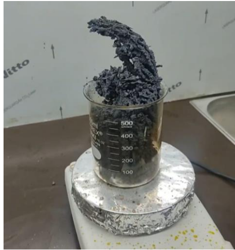
Figure 13 Displays the appearance of flameless auto-combustion.
