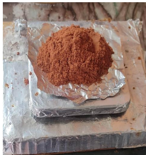
Figure 14 Mixed spinel ferrite powder after sintering
