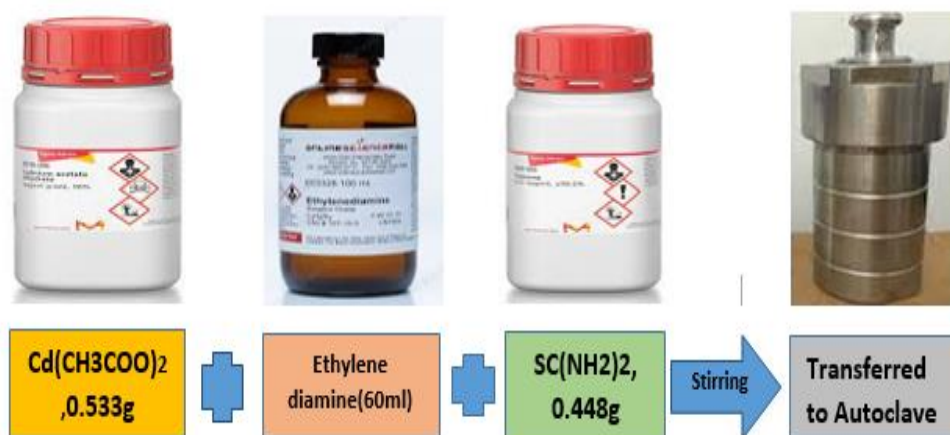
Fig.13: Flowsheet of CdS synthesis
